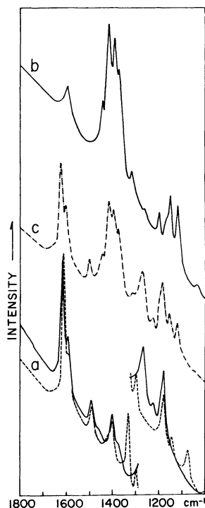
Fig. 1. Resonance Raman spectra of MO: (a) 1 \times 10^{-4} M in 0.1M HCl (solid line) and in 0.1M DCl (broken line), 514.5 nm; (b) 2 \times 10^{-4} M in water, 488.0 nm; (c) 2 \times 10^{-4} M in the phthalate buffer (pH 3.4), 488.0 nm.
